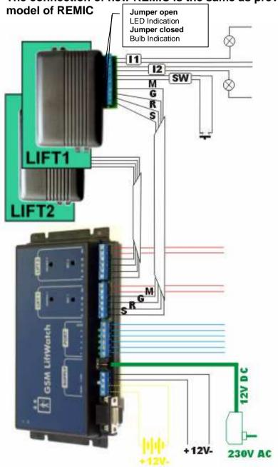
Example of connection – activation by galvanically isolated screws of 12V switch at new ReMic – connection to bell or Alarm.
