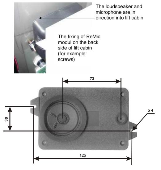
Fix the basic unit either on lift cabin or in machine room (neccessary when use it for 2 lift cabins). The GSM signal determine where basic unit is install. The installation on lift cabin is easier but you must verify that GSM signal is available during all lift way. Keep enough space for SIM card manipulation.
